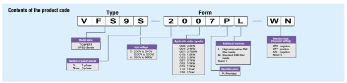
Note) 1. L:Standard model without optional filter conform to "EN55011 Group 1 Class A"
