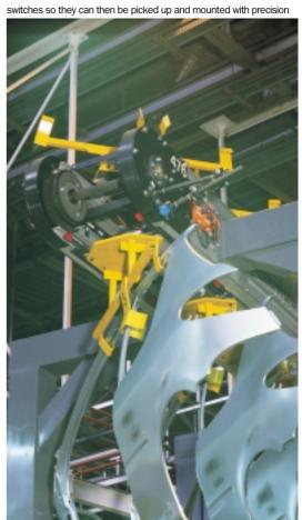
▼ Moulded sheet-metal parts used for the production of automobiles are detected with millimetre accuracy by WL 12 L-2 laser photoelectric
